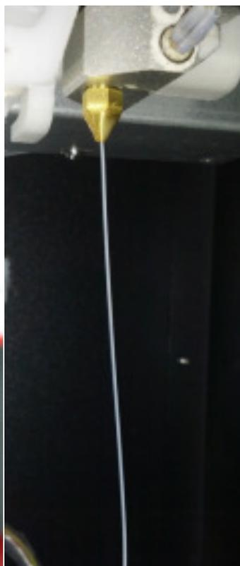
*Example of a good extrusion after doing an extrude.*
