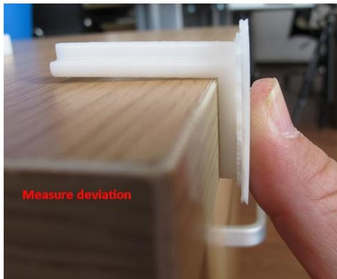
Remove the Front Centre ‘L’ shaped component, and measure its deviation. Put the exact value into the Z box. If it deviates to the right side, the value to be put into the Z box will be a positive value. If the deviates to the left, the value to put into the Z box will be a negative value.
