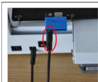
2. In the software, click 3D Print / Nozzle Height Detect. (if “Nozzle Height Detect” is greyed out check the connections)
