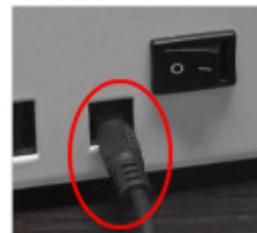
17. Plug in the black calibration cable into the auto levelling sensor and mount under the print head. There is a small hole in the print head cover where the sensor goes.
