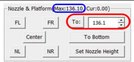
You will notice that the Max value has increased by 1mm. Repeat the above “Note 1” until the platform is 0.2mm away from the nozzle.
