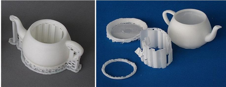
Printed models are composed of two parts. One part is the model itself, and the other part is the support material used to support any overhanging parts of the model.
