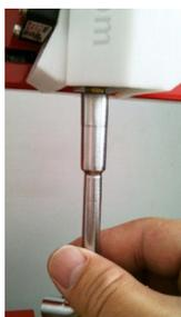
Should the nozzle become blocked, you may need to remove it in order to unblock. To remove the nozzle, first click **Withdraw** in the maintenance screen, then **only** once the printer is at 260c, use the nozzle wrench provided in the toolkit that comes with your UP Printer.
