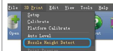
3. The table will rise up and the nozzle will touch the silver switch in order to automatically set the height. (the value will be around +/- 135mm)
