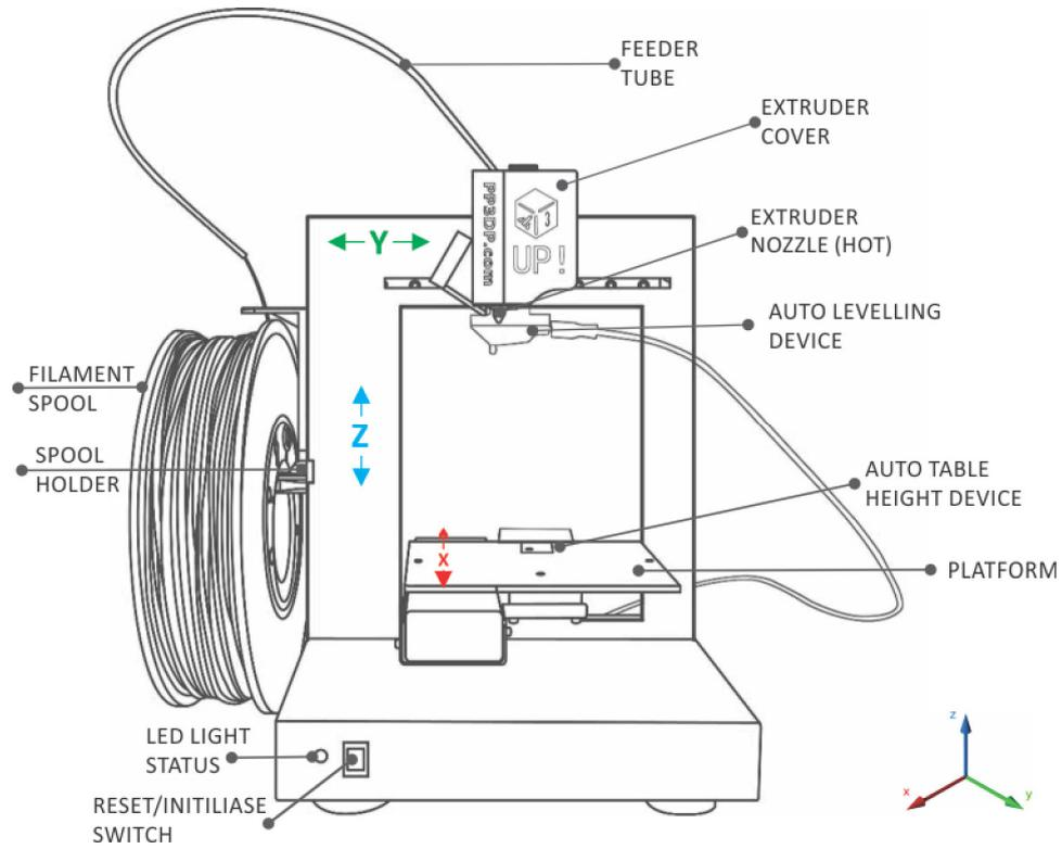
**Figure 2. Back view of printer**
